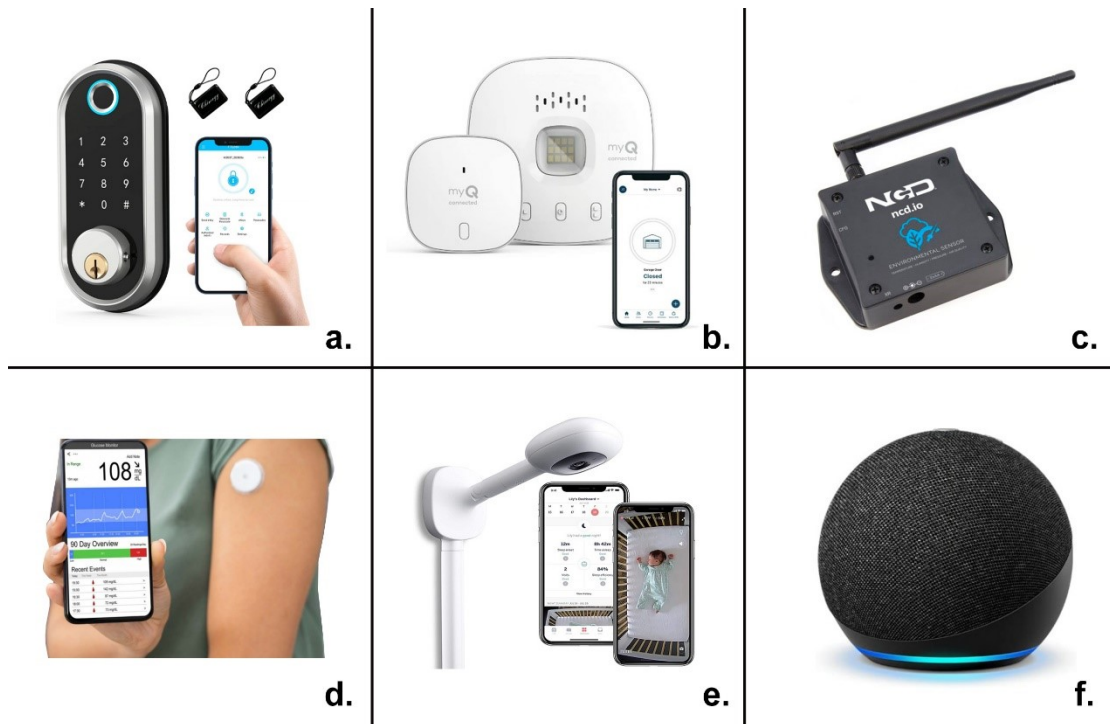
Figure 1: Examples of IoT devices: a. Smart Lock (Retrieved from here ); b. Smart garage control (Retrieved from here ); c. IoT wireless environmental sensor (Retrieved from here ); d. Glucose monitor system (Retrieved from here ); e. Smart baby monitor (Retrieved from here ); f. Smart Speaker (Retrieved from here )
