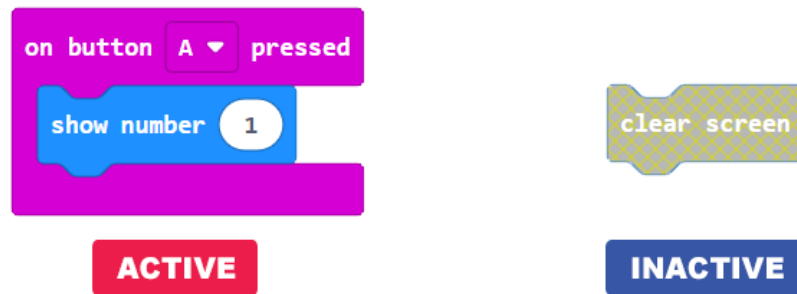
Figure 18: Examples of active and inactive scripts/codes. The clear screen command will not be executed
