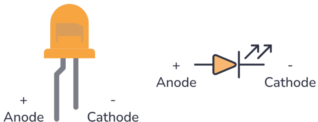
Figure 2.2: A LED with anode and cathode marked (left image) and a diode symbol (right image). Source: https://www.build-electronic-circuits.com/what-is-an-led/ .
